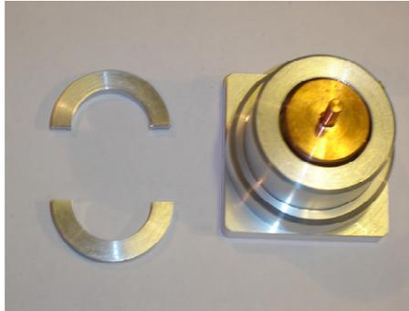
If the flux from the magnets is not perfectly homopolar, then the mechanical center and the magnetic center will be separated. Reasons for this are described in more detail in Chapter 5.6. The separation distance is a way to measure the quality of the magnets.
